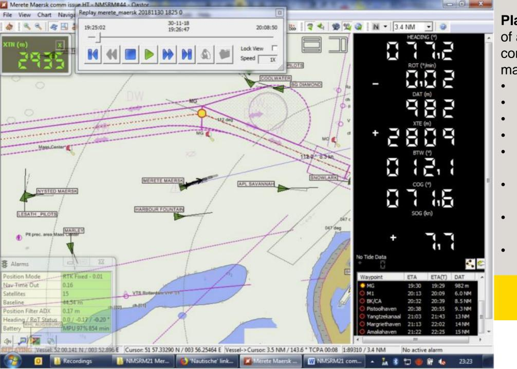
Planning port passage of a 400 m. long container ship by a maritime pilot, using:
